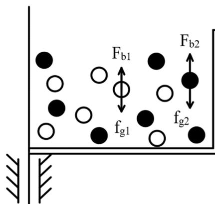
Figure 1a. The force on the ore particles when the equipment is stationary
