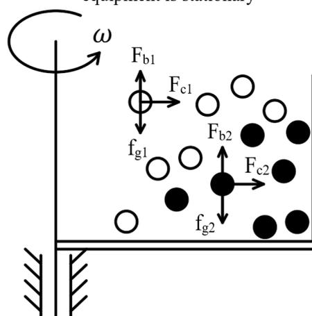
Figure 1b. Schematic diagram of the stress on the ore during reselection
