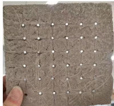
Figure 6. Concrete test block after grinding
