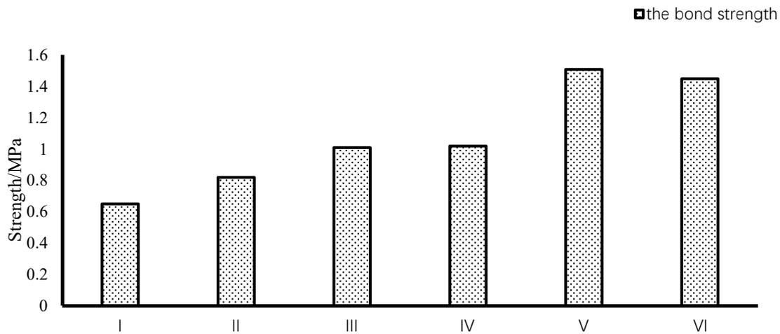
**Figure 7.** Bond strength between different matrix materials and acrylic
