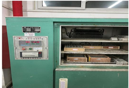
Figure 4. Concrete constant temperature steam curing box
