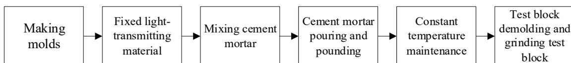
Figure 1. Test block production process
