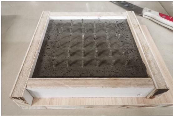
Figure 3. Schematic diagram of the mold (150×150×36)
