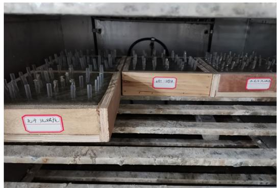
Figure 5. Specimen block in constant temperature steam maintenance
