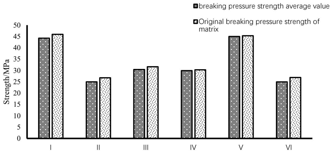
**Figure 8.** Compressive strength of different matrix materials combined with acrylic
