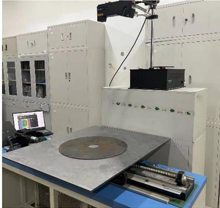
Figure 3. Skeleton plate flatness detection installation erection diagram
