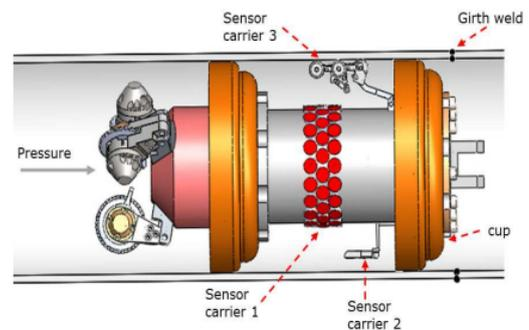
Figure 6. PIG robot
