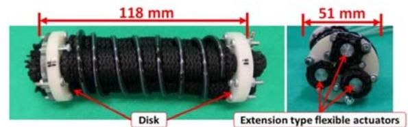
**Figure 13.** Flexible pneumatic robot
