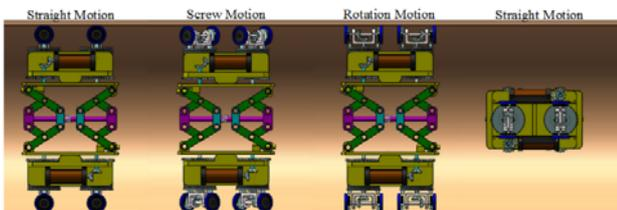
**Figure 8** Multi motion mode of screw driven robot
