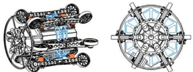
**Figure 3.** Multi link articulated wheeled pipeline robot
