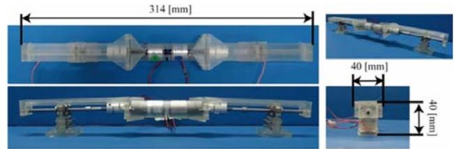
**Figure 12.** Inchworm robot
