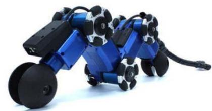
**Figure 2.** Multi link articulated wheeled pipeline robot
