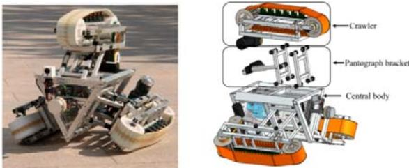
Figure 4. Multi link articulated wheeled pipeline robot
