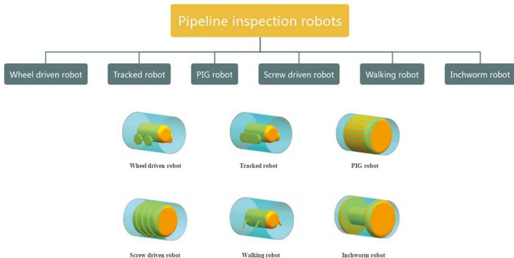
**Figure 1.** Classification of pipeline inspection robots
