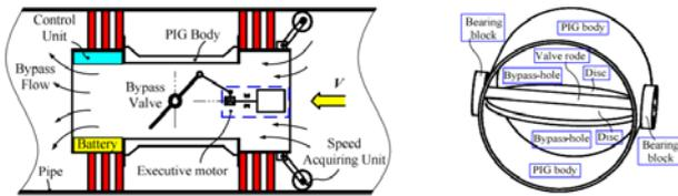
**Figure 7.** The structure of butterfly bypass valve speed regulating robot
