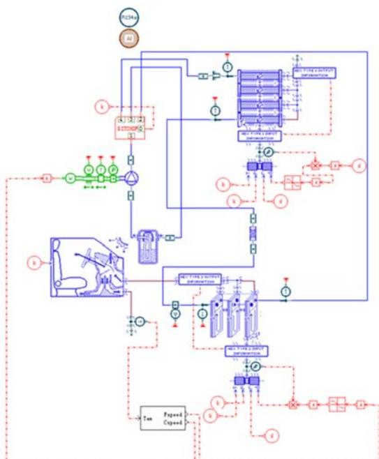
**Figure 7.** Simulation Model of Fuzzy Control AMESim for Heat Pump Air-conditioning
