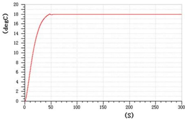
Figure 9. Temperature Rise Curve of Vehicle Indoor at Idle Speed
