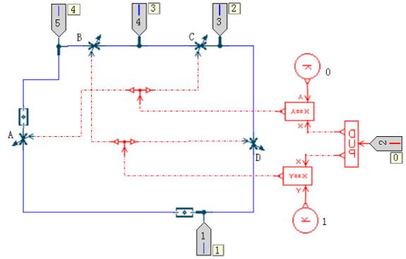
Figure 4. Four-way reversing valve model
