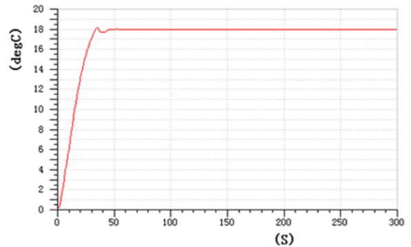
Figure 11. Simulated Temperature of Vehicle Room under Common Speed Conditions
