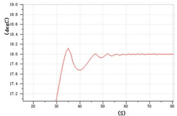
Figure 12. Local enlargement of simulated temperature in compartment under common speed conditions
