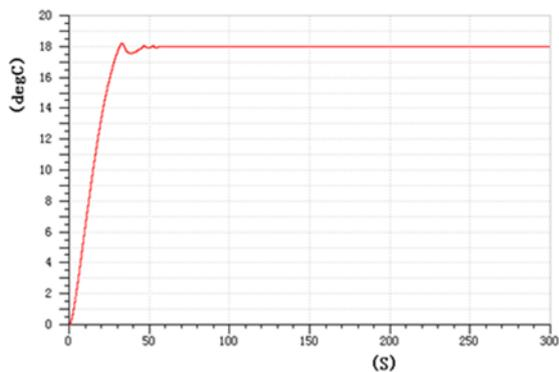
Figure 13. Simulation Temperature of Car Room under High Speed Conditions
