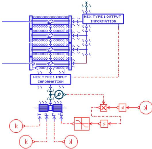
Figure 2. Outdoor tube-fin heat exchanger assembly model
