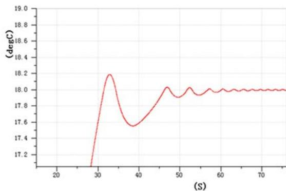
Figure 14. Local Amplification of Simulation Temperature in Car Room under High Speed Conditions
