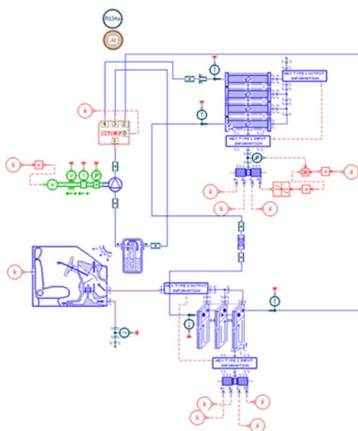
**Figure 6.** General simulation model of heat pump air conditioning system for electric vehicle
