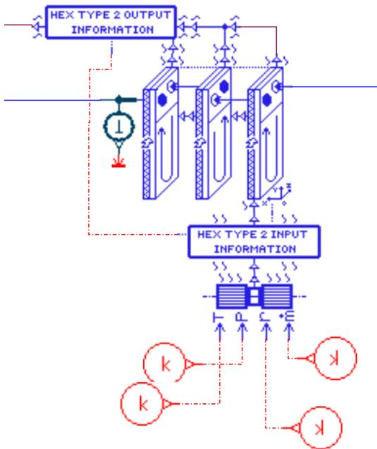
Figure 3. Indoor heat exchanger and fan assembly
