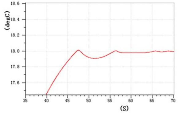
Figure 10. Local enlargement of indoor temperature rise curve at idle speed
