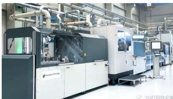
**Figure 2.** Blackstone Technology Battery 3D Printer
