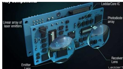
Figure 14. Example of flash method
