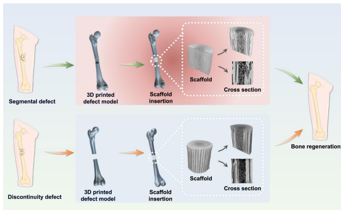
Figure 2. Schematic diagram of the manufacturing strategy for repairing personalized bone defects. The upper panel shows the case of a segmental defect, while the lower panel shows the case of a discontinuity defect.
