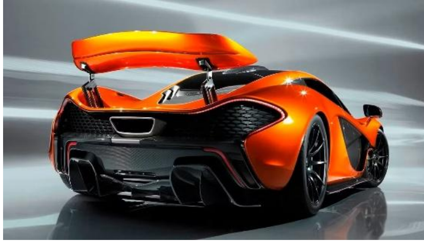
Figure 4. McLaren P1TM's rear spoiler (fully extended) [16].
