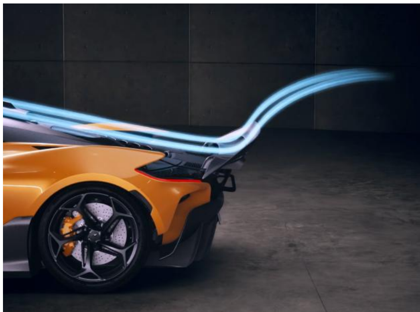
Figure 2. McLaren W1 Airbrake airflow [11]
