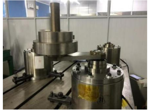
Figure 8. PI parameter tuning experimental device for variable moment of inertia
