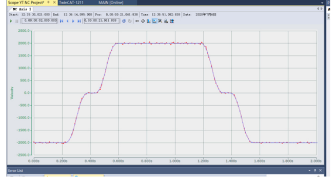
Figure 9. Speed fluctuation of traditional PI controller
