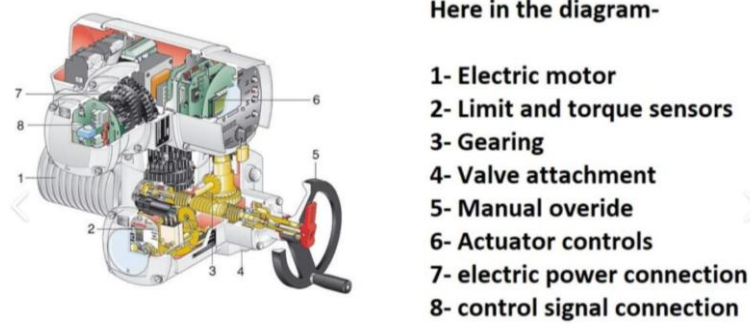
Figure 3. Electric valve actuators
