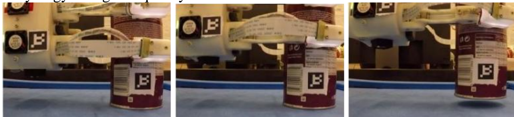
Fig. 2 Initial phase of grasping an object with tactile data [6]
