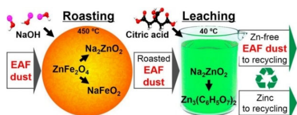
Figure 4. Schematic diagram of the mechanism of alkaline roasting and citric acid leaching [30]
