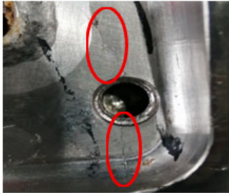
Figure 1. Crack initiation source and propagation direction of the threaded hole in the non-magnetic drill collar
