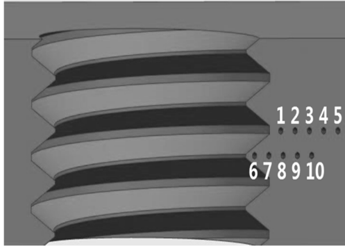
Figure 7. Schematic diagram of Vickers hardness indentation points
