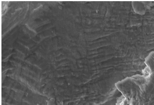
Figure 12. Fatigue striations of the extruded thread
