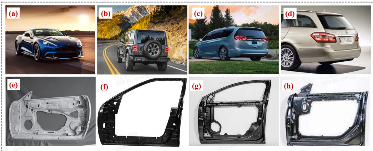
Figure 3. Development and application of Mg alloys in car doors: (a) Aston Martin Vanquish S with cast Mg side door inner; (b) All-new 2018 Jeep Wrangler produced with a die-cast Mg rear swing gate; (c) Chrysler Pacifica showing the liftgate assembly highlighted by a Mg die-cast inner; (d) The rear end of the Mercedes-Benz E-Class T-Model featuring the hybrid Mg-Al hatch back; (e) Inner door frame of the Daimler-Chrysler SL Roadster; (f) Ford’s concept die-cast Mg door inner with an open architecture; (g) Integrated Mg die-cast door inner designed as part of a DOE sponsored project led by GMC; (h) Ultra-thin and ultra-light Mg alloy door inner.
