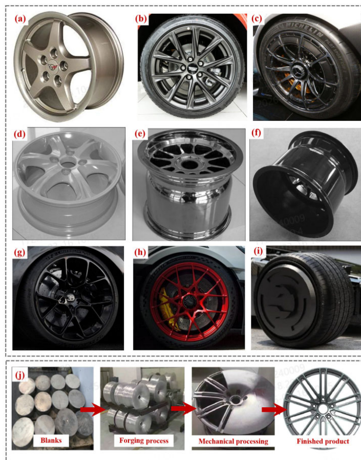
Figure 7. Mg alloy wheel applications and manufacturing processes: (a) Chevrolet Corvette low-pressure cast wheel; (b) Cadillac CT4-V forged-spun wheel; (c) AMG Project One bionic-design forged wheel; (d–f) AZ80 hollow-billet extruded wheels; (g) Bugatti Chiron Super Sport 300+; (h) Porsche 911 GT3 RS forged wheel; (i) Bandit9 electric racing wheel; (j) Forward-and-reverse extrusion forming process.
