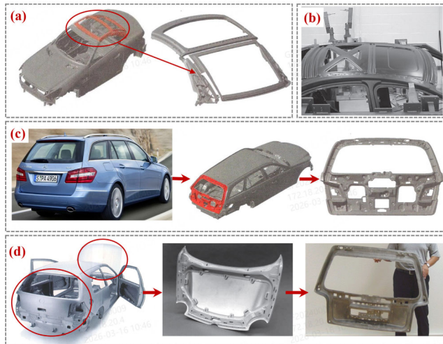
Figure 6. Mg alloy applications in roof panels, engine hoods, and trunk lids: (a) Mercedes-Benz SL/SLK series folding Mg roof; (b) Chrysler Mg-intensive body inner panel; (c) Mercedes E-Class touring trunk lid (AM50); (d) VW Lupo Mg trunk lid and hood prototypes.
