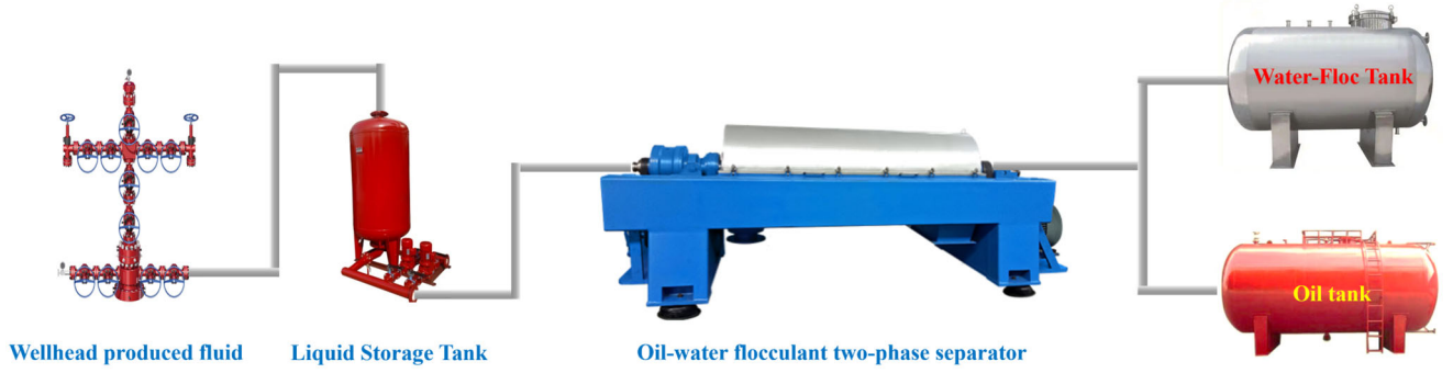
Figure 4. Process flow diagram
