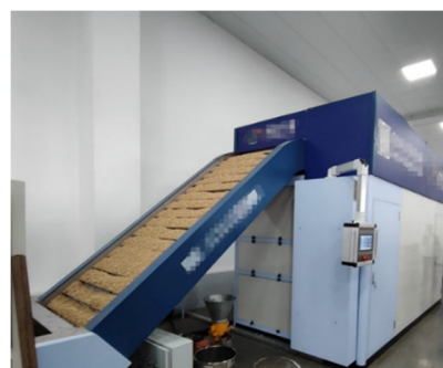
Figure 1. Mesh belt dryer
