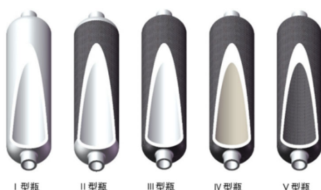
Figure 1. Structural forms and development of Type I to Type V hydrogen storage cylinders
