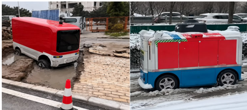
Figure 6. Traversal dilemmas of traditional ground inspection equipment on complex road surfaces
