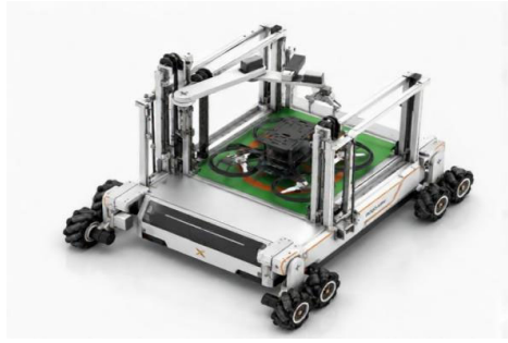
Figure 13. SCARA manipulator performing UAV inspection and maintenance tasks
