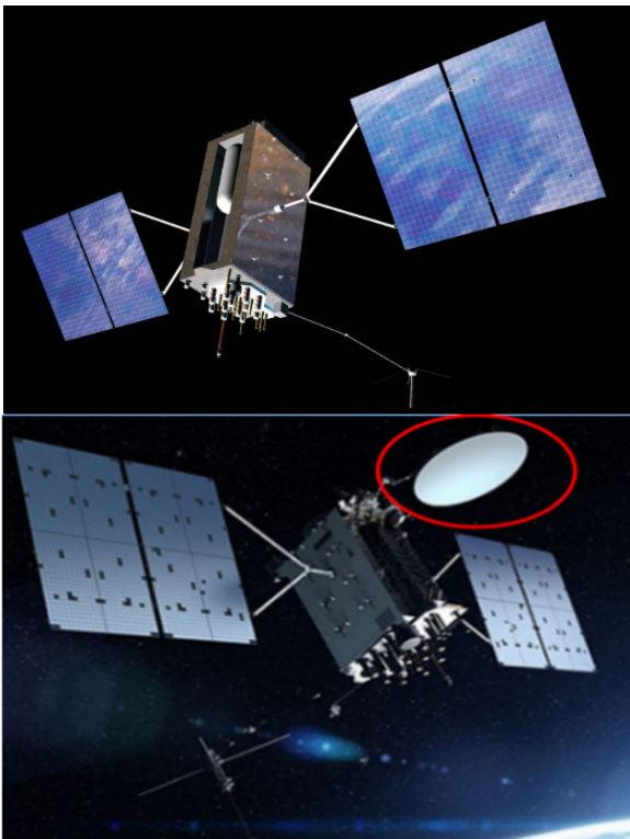
Figure 2. GPS-IIIA and GPS-IIIF Satellites (Power Enhancement Antennas Circled in Red)
