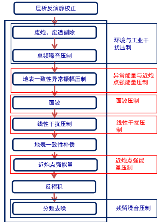
Figure 3. The flow of combined denoising technique before stacking with amplitude fidelity preservation
