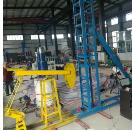
Figure 6. Pumping unit test system device
