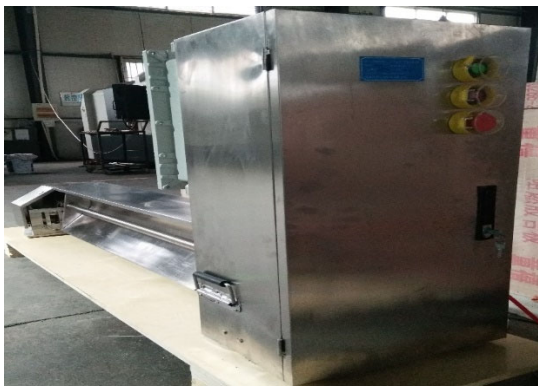
Figure 2. Cuttings weighing device
