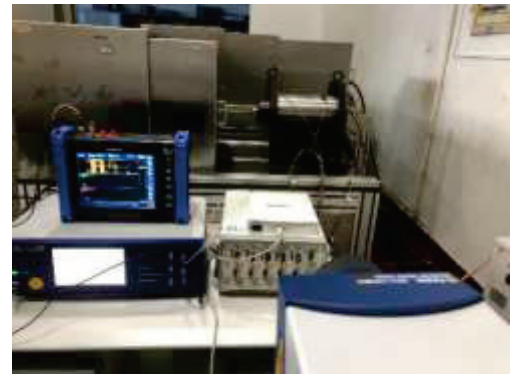
Figure 3. The vibration test diagram of spindle
