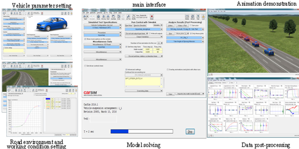
Figure 3. Function and interface diagram of CarSim
