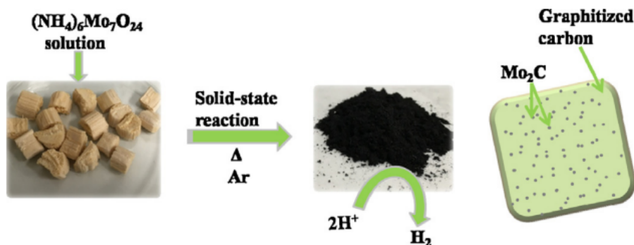
Figure 3. Schematic diagram of the preparation of biomass-based \text{Mo}_2\text{C}/\text{C} nanoparticles
