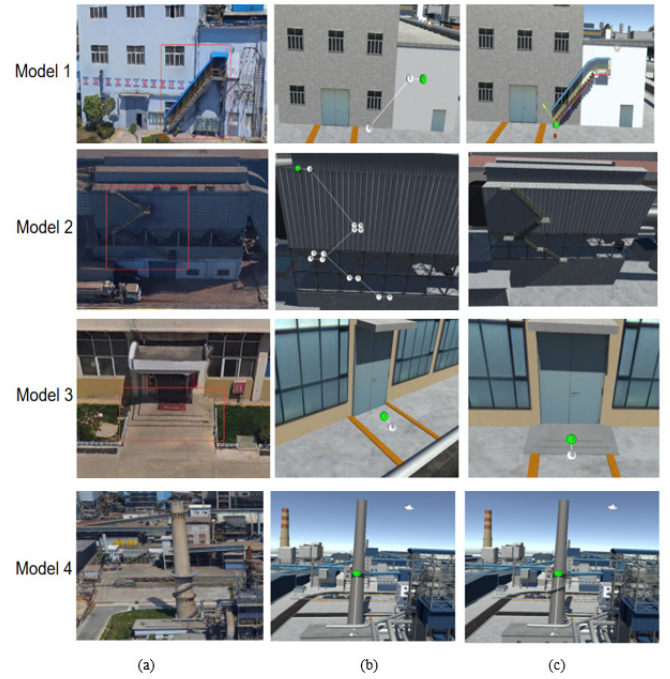
Figure 10. Shows an example model generated based on the framework curve, where (a) is oblique photography, (b) is the facility framework curve, and (c) is the output facility model
