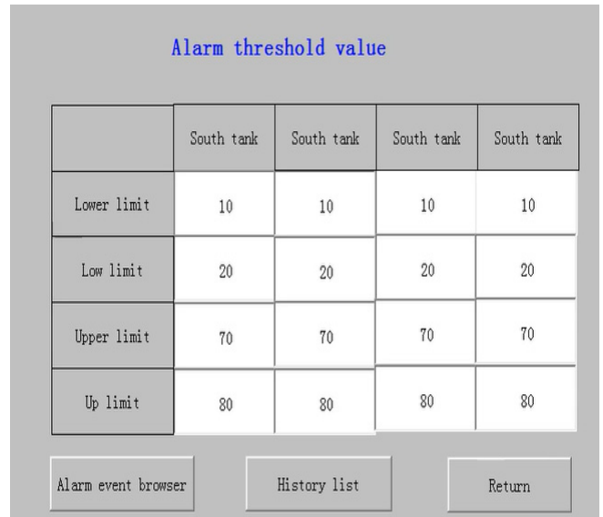
Figure 9. Alarm threshold setting
