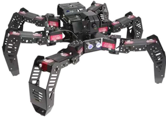
Figure 4. Intelligent inspection multi-legged robot
