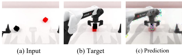
Figure 5. Comparative analysis of stack blocks task execution: (a) Original input sequence with uniform values, (b) RoboTwin-simulated target sequence, and (c) Model-predicted sequence after fine-tuning.
