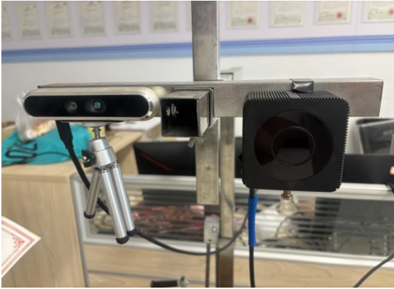
Figure 4. Joint calibration model between camera and 3D LiDAR
