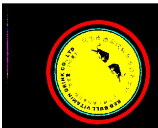
Figure 5. Segmentation Map of Printed Connected Domains on Tank Cover
