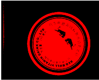
Figure 4. Threshold Segmentation Map for Tank Cover Printing
