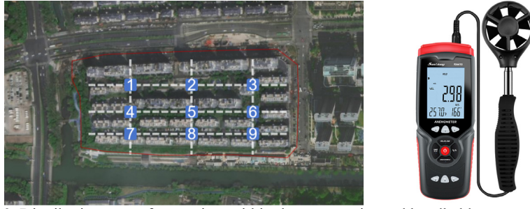
Figure 2. Distribution map of test points within the community and handheld anemometer GM8902+
