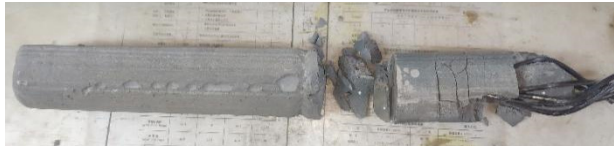
Fig 8. Damage of grout cement in bamboo tube
