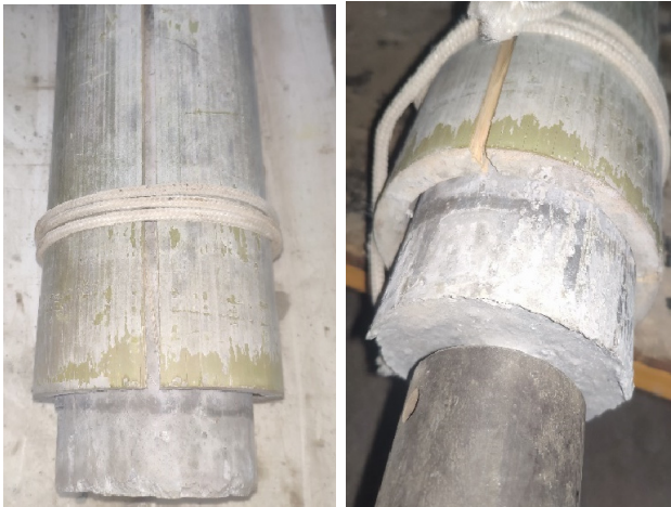
Fig 13. Example of tensile damage of short steel sleeve specimen
