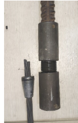
Fig 6. Structural schematic and solid diagram of threaded steel strand adapter
