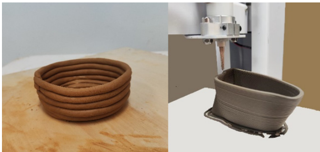
Fig 2. Ceramics made with panning clay strips and 3D printing
