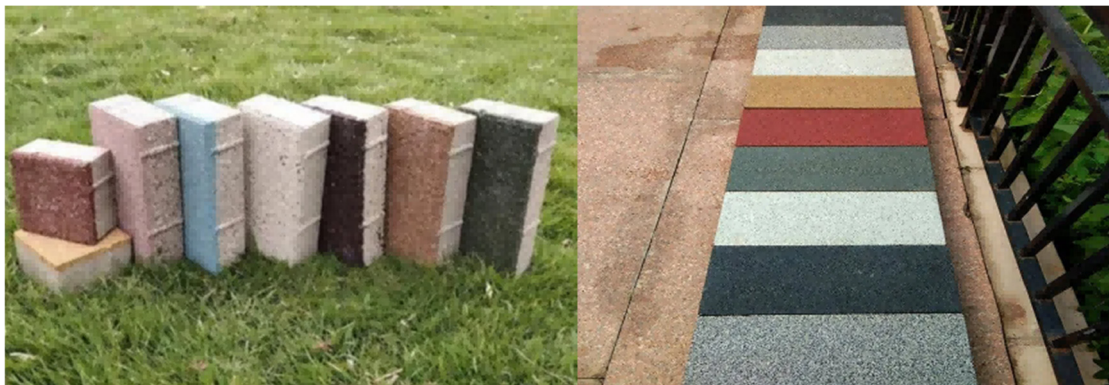
Figure 4. Permeable bricks made of artificial stone recycled from construction waste
