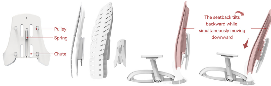
Figure 5. Sliding Back Component and Backrest Movement Description
