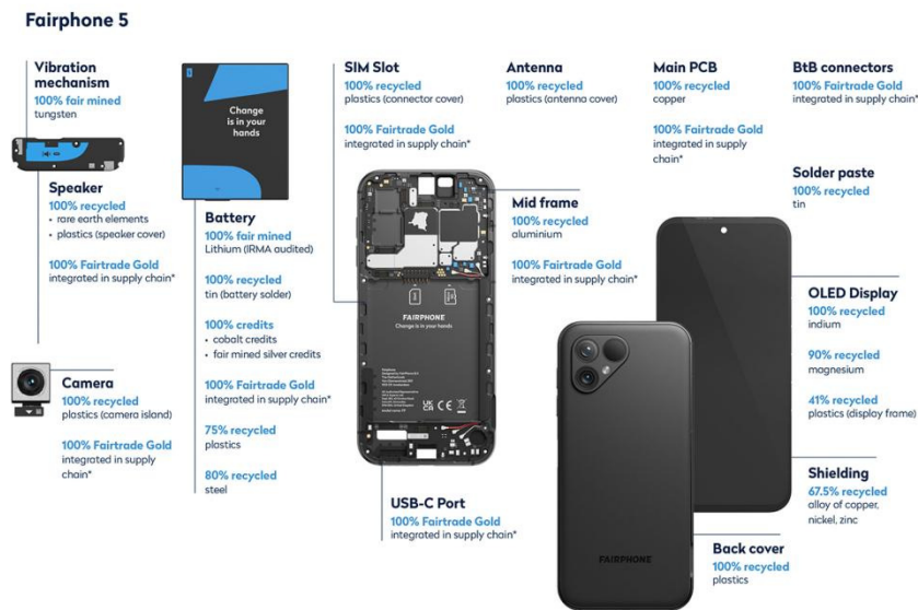
Figure 1. Disassembly structure of Fairphone 5
