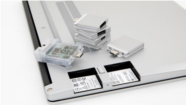
Figure 3. Modular interface design of Framework Laptop
