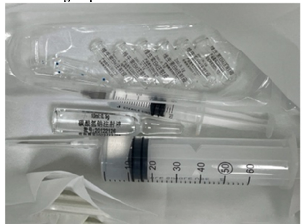
Foaming test items: Foaming test article: 6 pieces of vitamin B6 2ml solution, 1 piece of 5% sodium bicarbonate 10ml solution, 1 piece of 50ml syringe and 5ml syringe.
