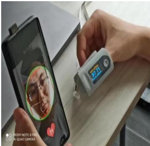
Figure 13. rPPG was consistent with heart rate measured by finger clip
