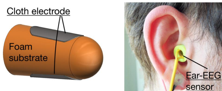
Figure 2. An in-ear EEG sensor with a generic earpiece. The left part of the picture shows a close-up view of the earpiece with two flexible electrodes. Right diagram illustrating the sensor's placement within the ear canal [14]
