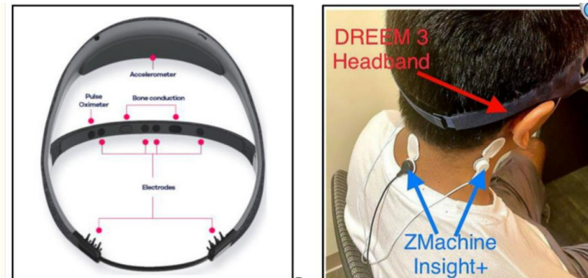
Figure 1. The Dreem Headband (DH): (left) Sensor configuration schematic; (right) Simultaneous EEG signal recording comparing the DREEM 3 and Zmachine Insight+ systems [12]
