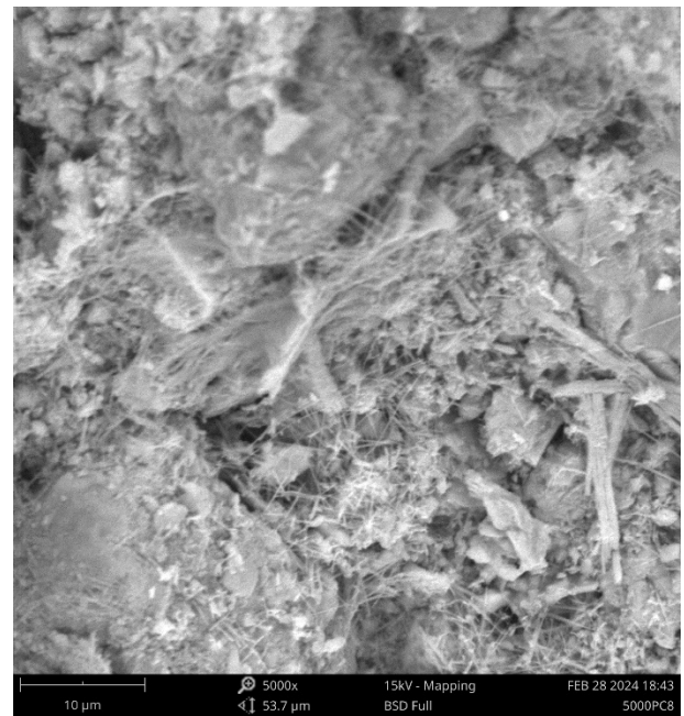
Figure 5. Micro-morphology of RCP cured soil
