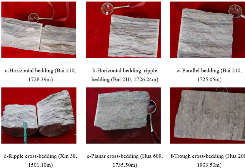
Fig 9. Layered structural characteristics of Chang 3 sandstone in the Baibao area
