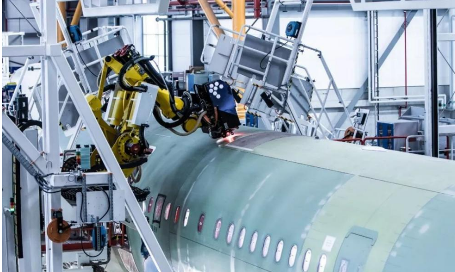
Figure 1. Robot automatic drilling (aircraft assembly)
