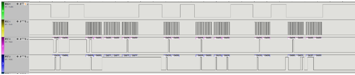
Fig. 11 Timing diagram of RT address enablement in FPGA version
