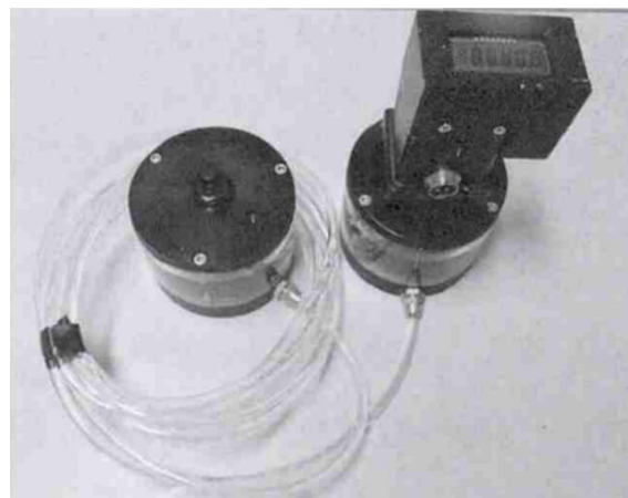
Figure 7. Differential air pressure type high accuracy vertical displacement sensor [19]
