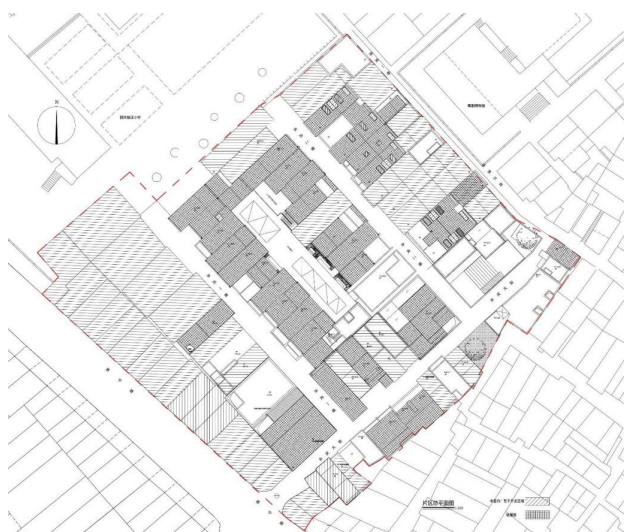
Figure 3. General plan of Yongqingfang after renovation (data source: Guangzhou Vanke Yongqingfang Project Department)
