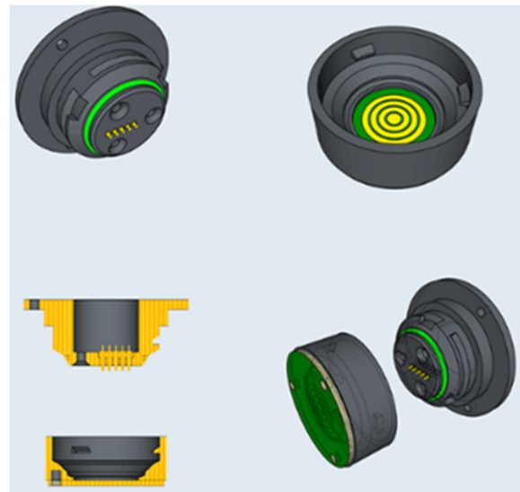
Figure 3. Schematic diagram of sensor mechanical interface design
