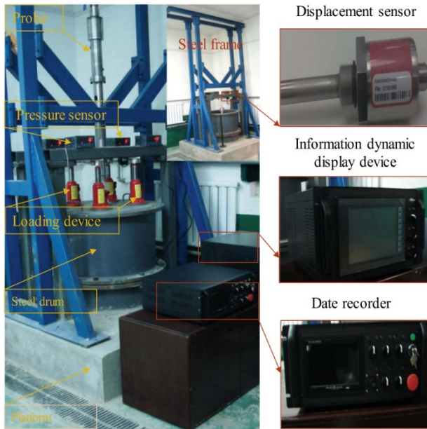
Fig 6. Main instruments of in-situ borehole pressure shear test [75]
