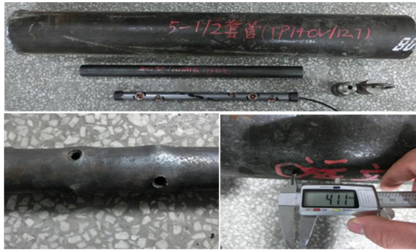
Figure 5. Testing Perforator and Post Perforation Gun and Sleeve Status
